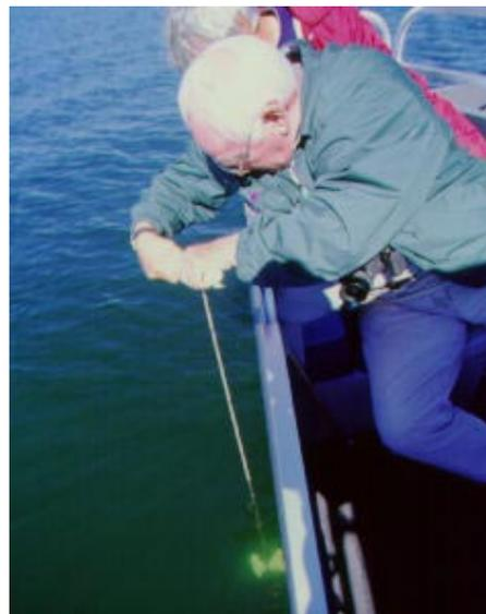
4. When the secchi disk just disappears from view, mark the rope at the water level with a clothespin.
